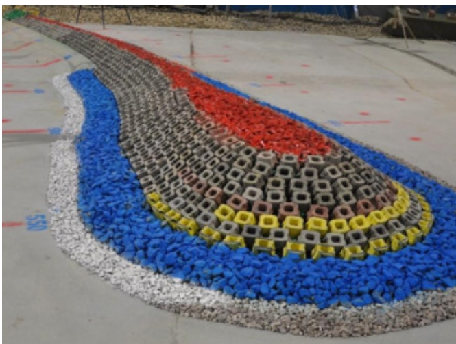
Physical model of a coastal structure tested in a laboratory wave flume
